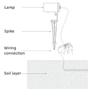
b. After matching the position, the Luminaire and the pre-embedded power cord wiring are wrapped and waterproofed, and then press the spike into the mud layer from top to bottom to fix it firmly. (After completing the installation, turn on the power.)
